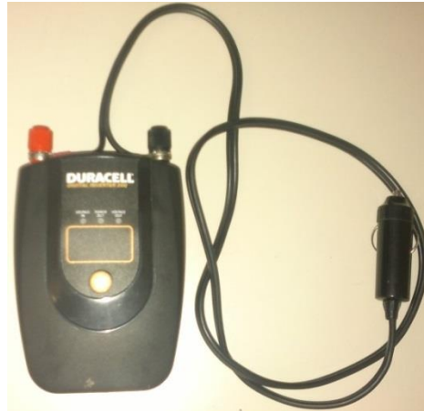
Figure 3. Inverter that helps to supply power from vehicles to the RFID system and associate computer when the tests are conducted inside vehicles.
