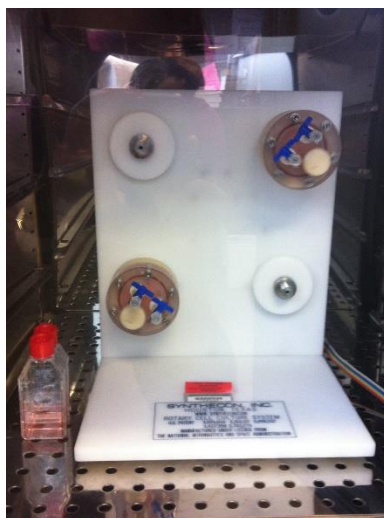
Figure 1. The High Aspect Rotating Vessel (HARV) simulating a microgravity environment. The vessel contains Jurkat cells in RPMI media.
