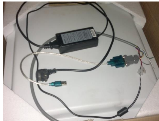
Figure 2. White rectangular receiver of the passive RFID system with connection cable to computer via USB port and a power adaptor for the operation of the receiver.
